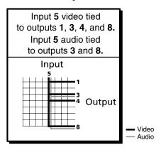
Figure 3-22 — Example 3, final configuration, audio switcher
